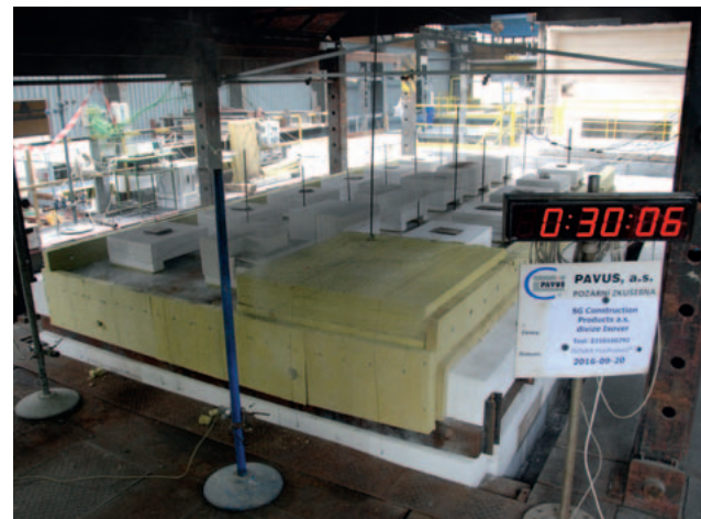
Fig. 10 Sample after 30 minutes - fire protection system ISOVER FireProtect® fulfils its function for 100 %, roof is without any deformation (bending stress, the same as would be under cold conditions)
