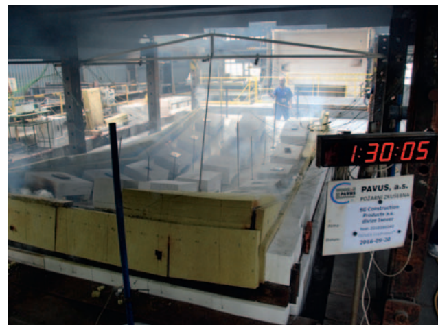
Fig. 11 Sample after 90 minutes - roof deformation protected with ISOVER FireProtect® is close to limit deformation given by test standard EN 1365-2 (fluent transition from bending stress to membrane)
